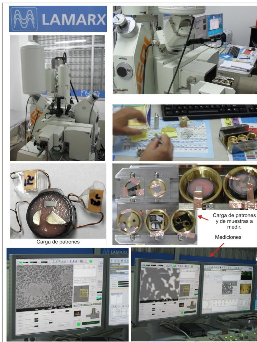
Figura 4-10: Microsonda JEOL JXA-8230. FaMAF, UNC.
