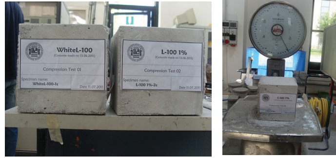
Figure 2.7: SFRC samples tested in compression.
